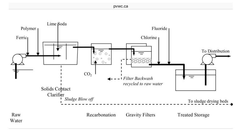
Upon entering Stanley's reservoirs, the treated water is re-chlorinated to ensure that required disinfection residuals are maintained throughout the system. Treated water is then pumped throughout the distribution system to the final consumer.
